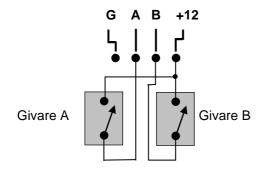
Suggestion for connection of alarm detectors in Normally Closed (NC) mode
